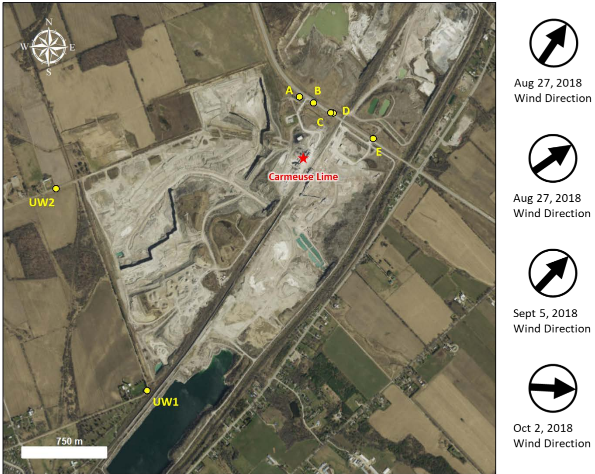
Figure 1: Locations of stationary half-hour measurements near Carmeuse Lime Beachville Operation (Ingersoll), August 27-28, September 5, and October 2, 2018. The arrow denotes the direction the wind was blowing during sampling dates. Sites UW1 and A, B, C, D are where TD tube samples were collected, UW2 and E are where the APCI/APPI TAGA unit measurements were made, and UW1 and C are where PM and TSP measurements were made.
